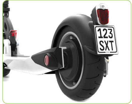
Brushless hub motor in rear wheel / Auto Power Off function
