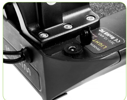
battery charging socket
